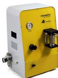
Fig. 2. A schematic of the helium porosimeter device
