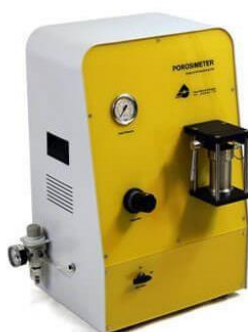
Fig. 2. A schematic of the helium porosimeter device
