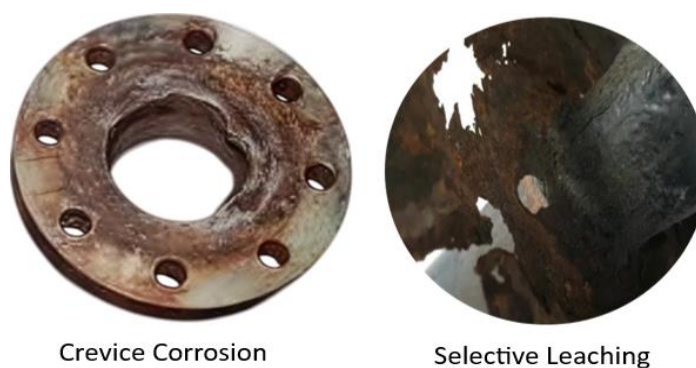
Fig. 8. Crevice corrosion and selective leaching [98, 100]
