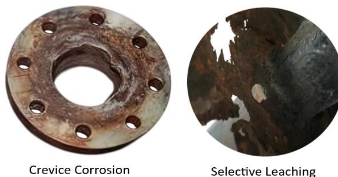
Fig. 8. Crevice corrosion and selective leaching [98, 100]
