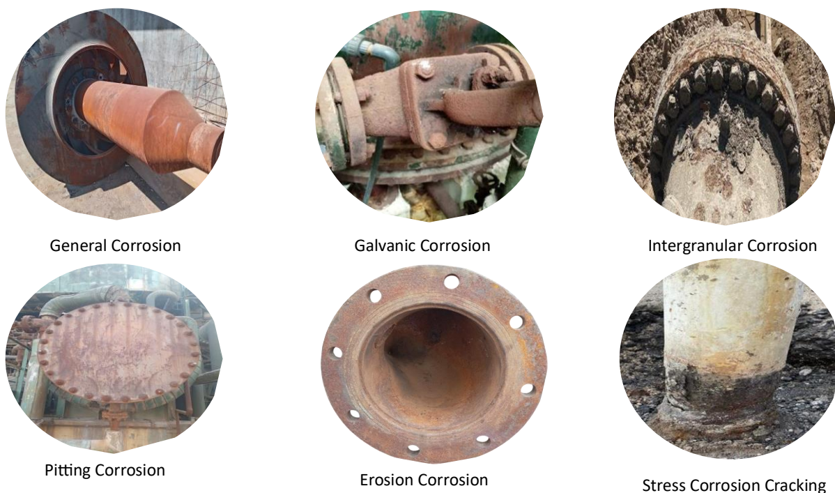
Fig. 7. Different corrosion patterns in carbon steel manufactured parts as observed at the thermal power station and refinery of Al-Dora-Baghdad, Iraq
