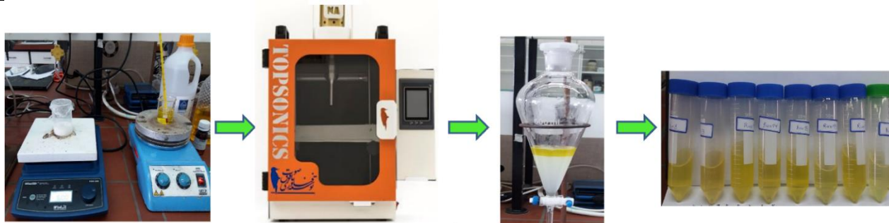
Fig. 1. Various stages of biodiesel production, separation, and purification
