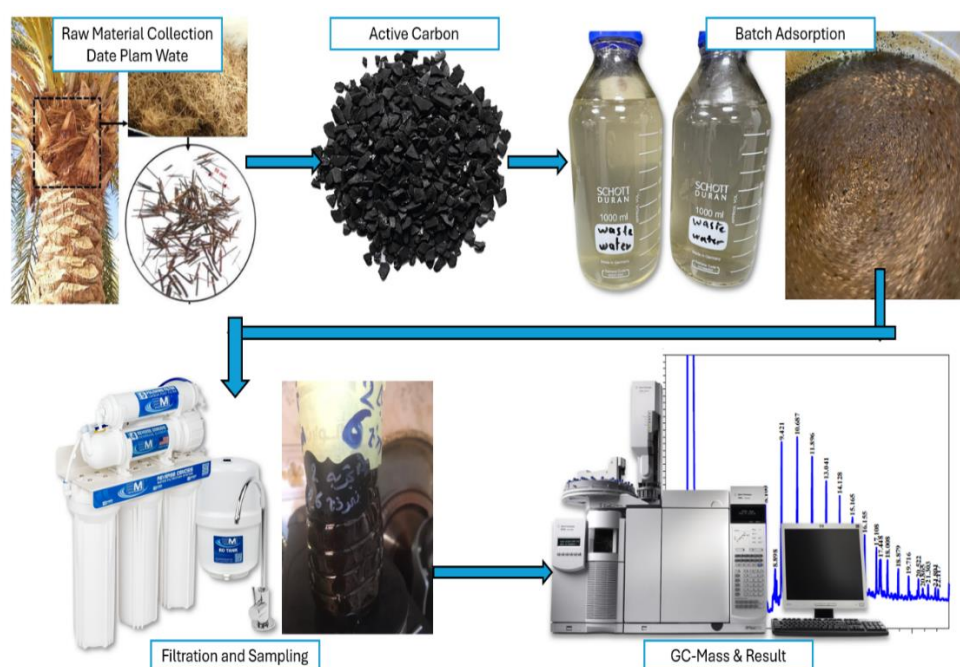
Fig. 3. Experimental workflow: Raw material collection and activation, batch adsorption (1.0 g in 500 mL, 90 minutes), post-treatment filtration and bottle sampling, and GC-MS analysis for PAH quantification
