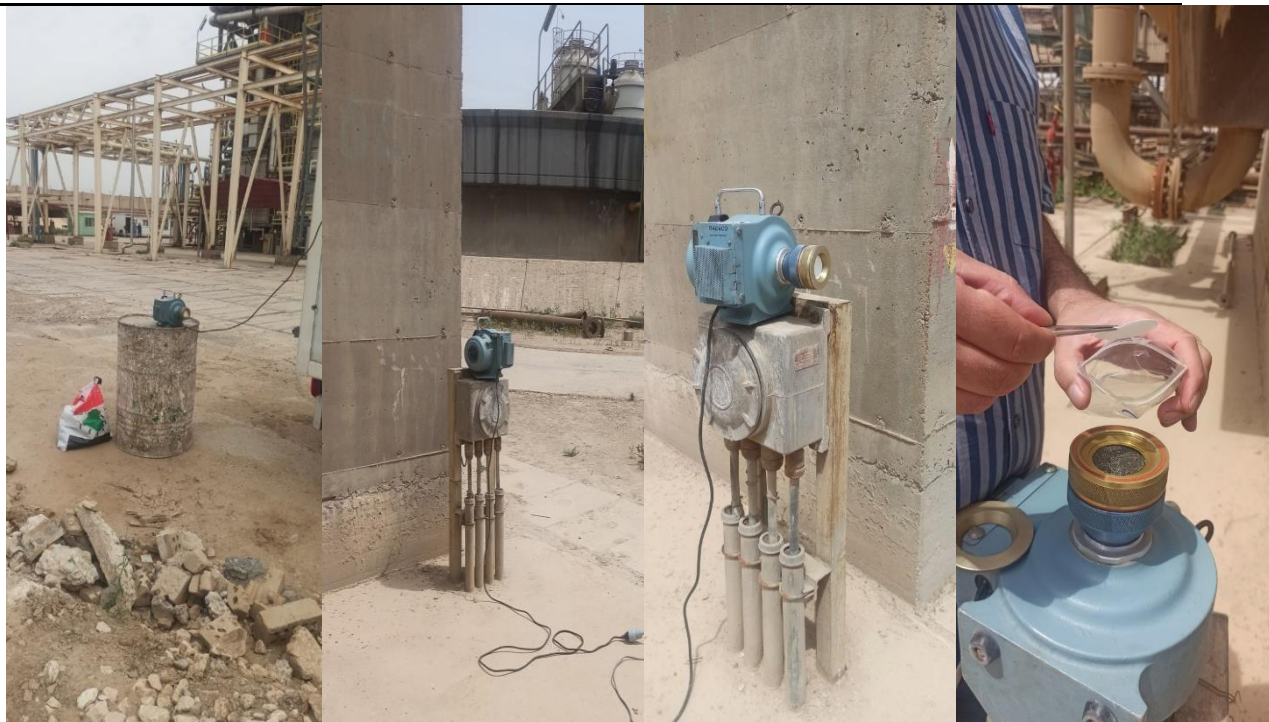
Fig. 4. Air sampling in Dora refinery
