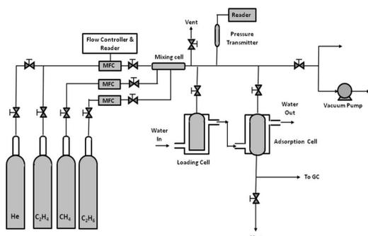
**Figure 2: Dynamic adsorption apparatus**
