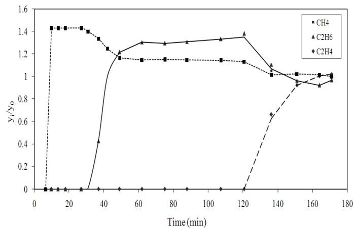
Figure 8: Adsorption breakthrough curves of methane, ethane and ethylene at 308.15 K.
