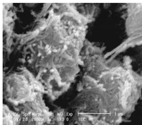
**Figure1: The SEM image of the prepared 10X zeolite**
