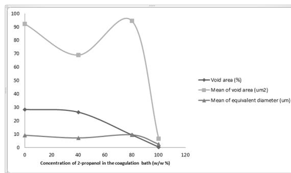
**Figure 12.** Void area (%), mean of voids area and mean of circle equivalent diameter of polyimide-based SRNF membranes against concentration of 2-propanol in the coagulation bath [142].
