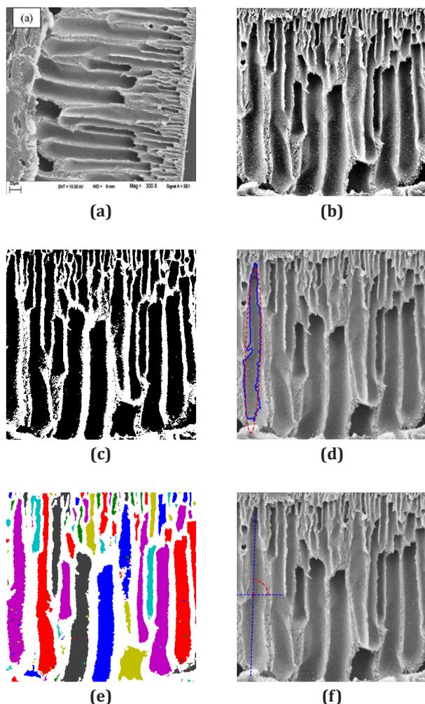
**Figure 7.** SEM analysis of polyethersulfone SRNF membrane in different stages of image processing: a) original image, b) pre-processed image, c) thresholded image, d) Boundary of void and fitting ellipse on original image, e) colorized voids, f) Orientation of the void (88.3°) [21].
