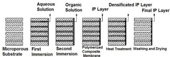
**Figure 5.** Schematic diagrams of the preparation process of TFC membranes by conventional IP technique [117].
