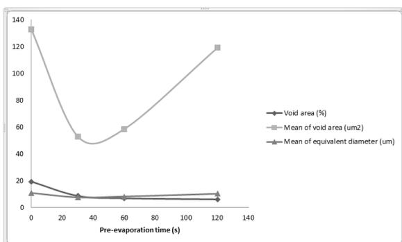
**Figure 11.** Void area (%), mean of voids area and mean of circle equivalent diameter of polyimide-based SRNF membranes against pre-evaporation time [142].
