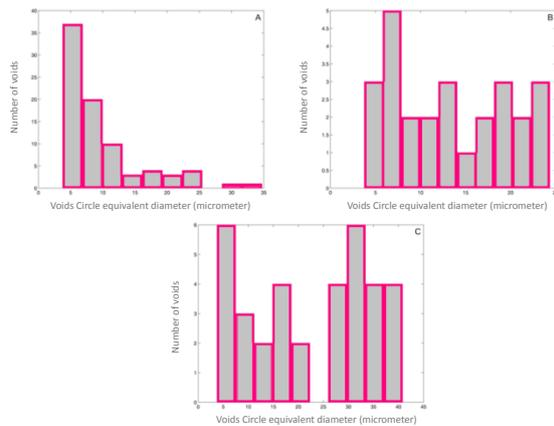
**Figure 13.** Population histogram of voids in different polymer concentrations in NMP as solvent: A) 15% B) 17% C) 23% [142].
