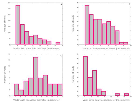
**Figure 15.** Population histogram of voids in different air velocities in pre-evaporation step: A) 0s B) 30s C) 60s D) 120s [142].
