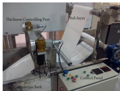
**Figure 2.** A pilot plant automatic instrument for phase inversion membrane preparation.
