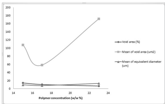
**Figure 9.** Void area (%), mean of voids area and mean of circle equivalent diameter of polyimide-based SRNF membranes against polymer concentration [142].
