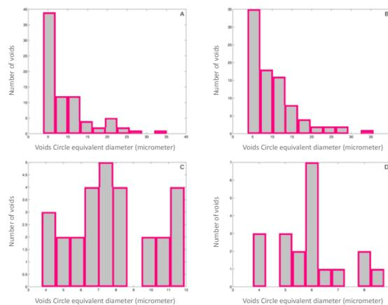
**Figure 14.** Population histogram of voids in different volatile co-solvent (THF) concentrations in the casting solution (base solvent was NMP): A) 0% B) 20% C) 60% D) 80% [142].
