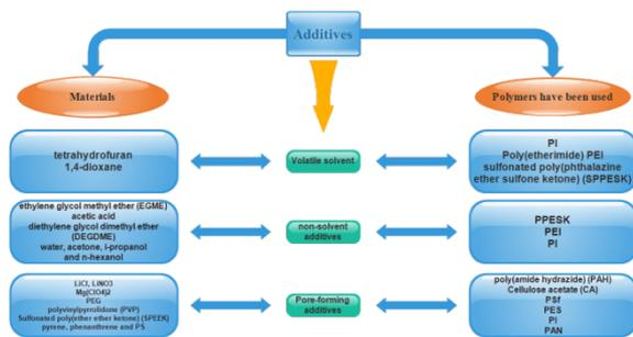
**Figure 3.** Additives for preparation of SRNF membranes casting solution [64, 88, 99-104].
