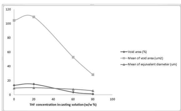
**Figure 10.** Void area (%), mean of voids area and mean of circle equivalent diameter of polyimide-based SRNF membranes against THF concentration in casting solution [142].
