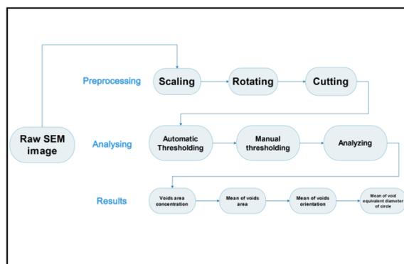
**Figure 8.** Whole SEM images computing with image processing process.
