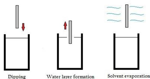
**Figure 4.** Dip coating method for preparation of TF on the sub-layer.
