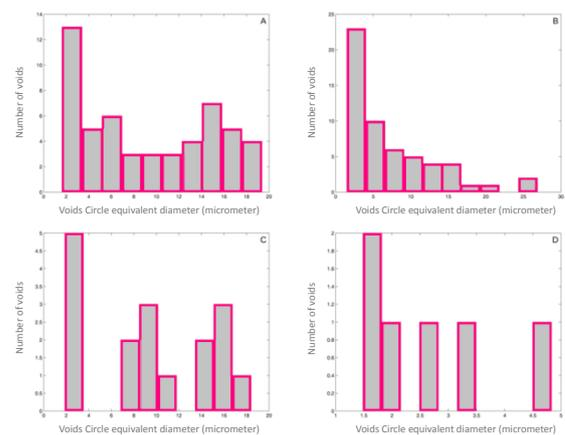
**Figure 16.** Population histogram of voids in different 2-propanol concentrations in the coagulation bath: A) 0% B) 40% C) 80% D) 100% [142].
