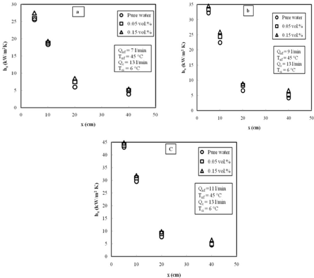
Fig. 3. Local heat transfer coefficient variation of  $\gamma$ -Al<sub>2</sub>O<sub>3</sub>/water nanofluid along axial distance at  $T_{nf} = 45$  °C, a)  $Q_{nf} = 7$  l/min, b)  $Q_{nf} = 9$  l/min, c)  $Q_{nf} = 11$  l/min
