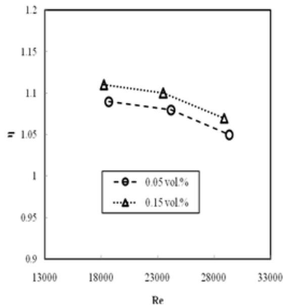
**Fig. 5.** Evolutions of thermal performance factor of the test section.
