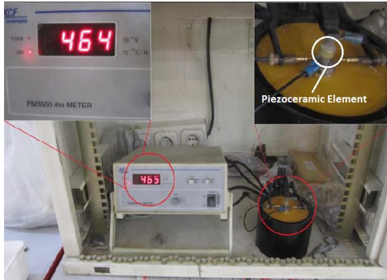
Fig. 3. Test setup for electrical impedance measurements
