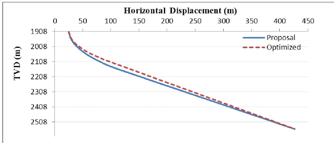
**Figure 6: Comparison between proposed & optimized well path**
