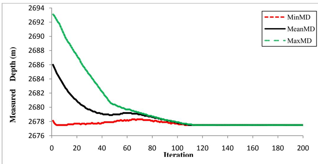
Figure 9: the highest, the mean value, and the lowest measured depth at each step. Convergence of particle swarm algorithm which results to find the shortest path is completely evidence.
