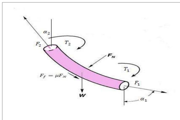
Figure 2: Drill string in curved section
