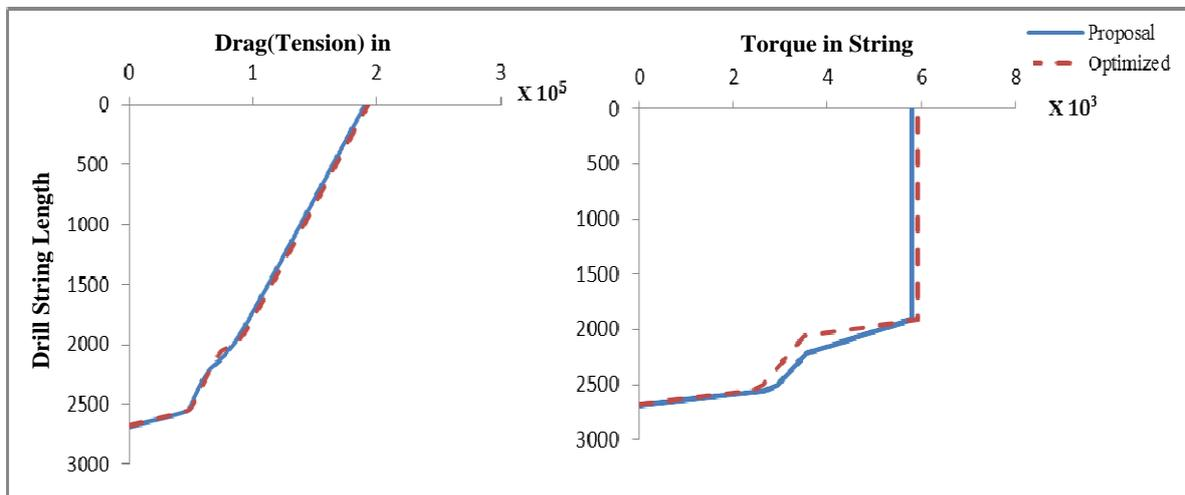
**Figure 7: Torque & Drag in drill string, comparison between proposed & optimized well path.** *In this case difference is negligible so choosing the proposed well path due to its lower drag and torque is not considered as an advantage.*
