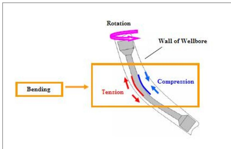
Figure 3: Forces exerted to drill string in curve section
