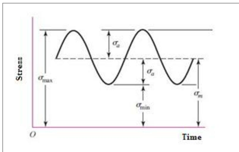
Figure 4: Stress-Time relation, fluctuating stress[8]
