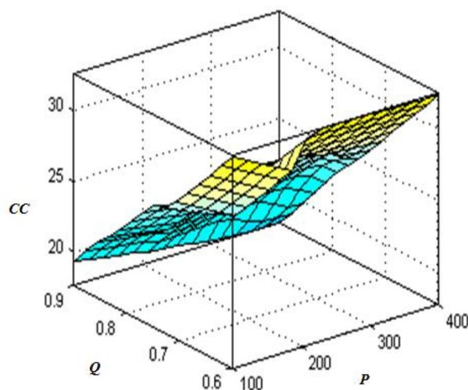
Fig. 7. Simulated response surface of Q, P, and cutting concentration for a state that  $T=125$ ,  $V=4$ ,  $RPM=60$ ,  $e=0.39$
