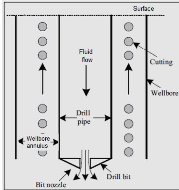
Fig. 1. Schematic of cuttings transport in a vertical-section
