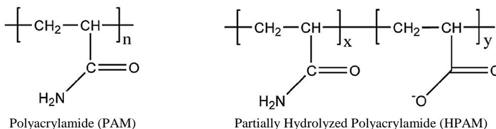
Fig. 2. Molecular structure of PAM and HPAM
