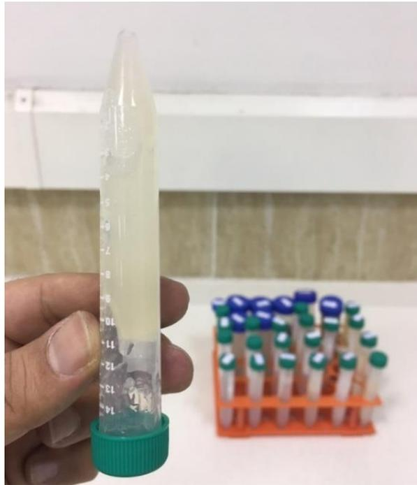
Fig. 5. Qualitative measurement of gel strength
