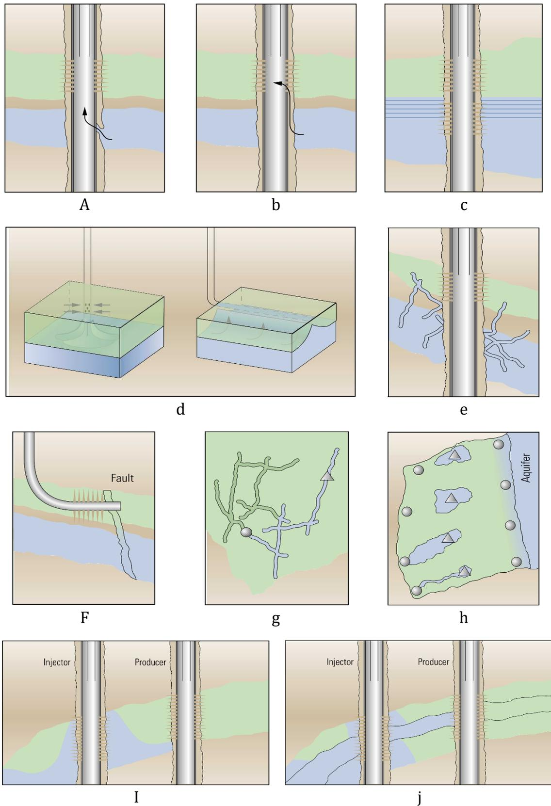
Fig. 1. Causes of water production in wells [1]
