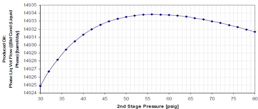
**Fig. 3.** The effect of 2<sup>nd</sup> stage separator pressure variation on the oil production rate, based on the transfer of 15% of Case#1 crude oil to the third stage separator with a pressure of 0.14 MPa
