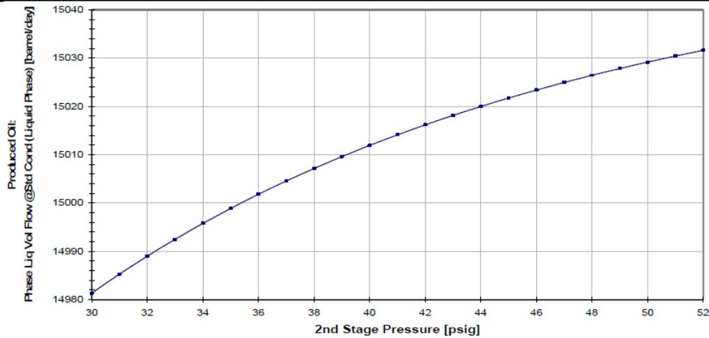
**Fig. 2.** The effect of 2<sup>nd</sup> stage separator pressure variation on the oil production rate, assuming the 3<sup>rd</sup> stage separator pressure be 0.14 MPa
