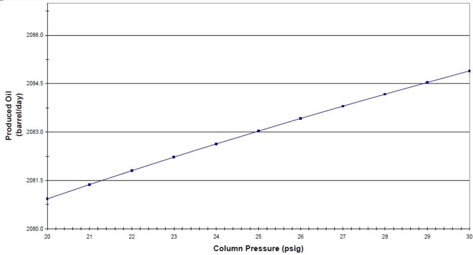
**Fig. A.10.** Effect of the column pressure variation on the oil production rate
