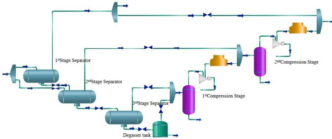
**Fig. A.7.** Schematic of crude oil production plant: The third method
