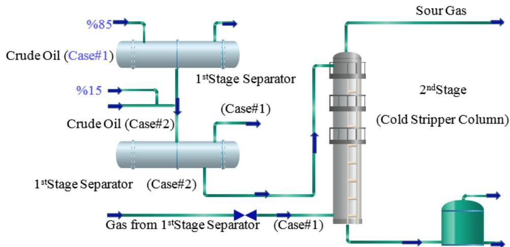
**Fig. 6.** The schematic of a crude oil production plant for case#1 and case#2 in a mixed-state
