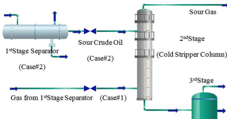
**Fig. A.9.** Schematic of crude oil production plant for case#2: Three separation stages
