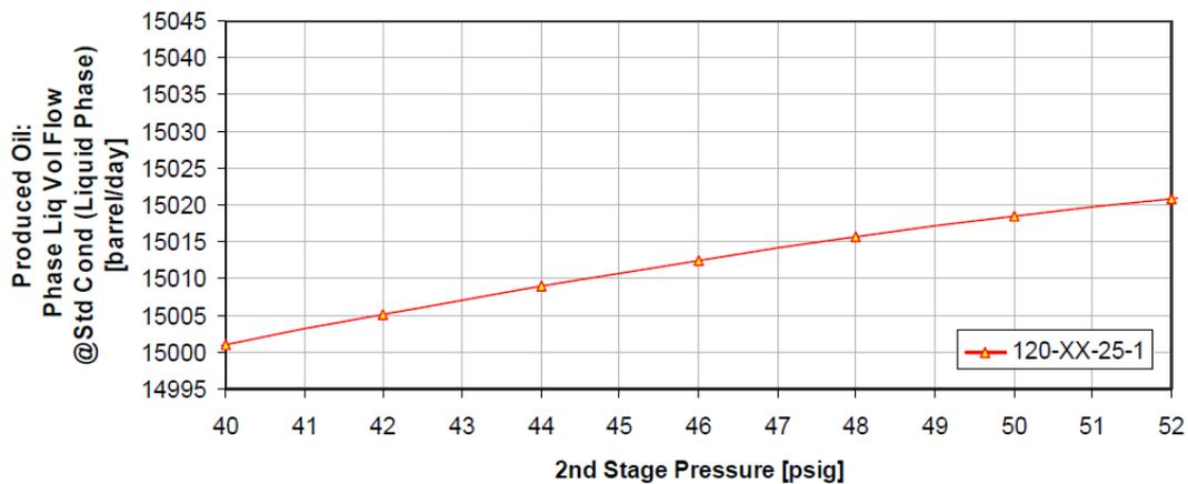
**Fig. A.2.** Changes in the Case#1 oil production rate versus 2<sup>nd</sup> stage separator pressure, assuming the 3<sup>rd</sup> stage separator pressure be 0.18 MPa
