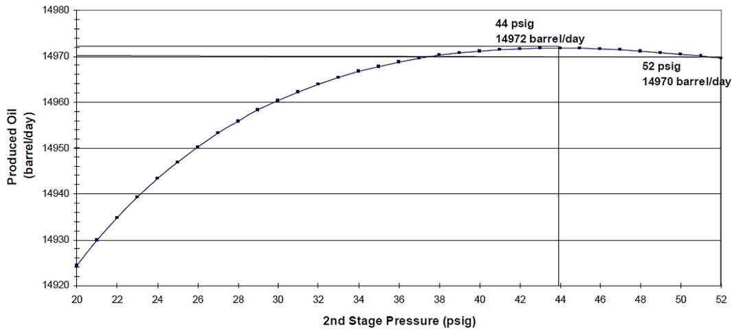
**Fig. A.4.** Effect of 2<sup>nd</sup> stage separator pressure variation on the oil production rate
