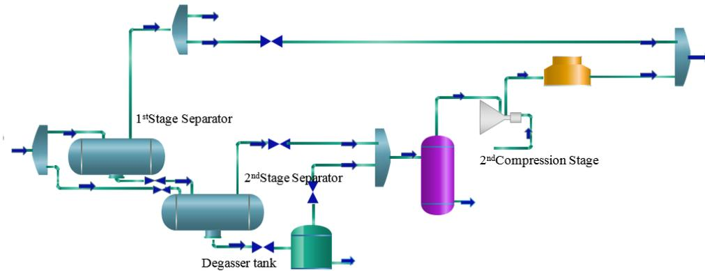
**Fig. A.8.** Schematic of crude oil production plant: an alternative for collection of gases from three stages of separation
