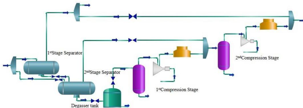
**Fig. 5.** The schematic of crude oil production plant: Collection of gases from three stages of separation
