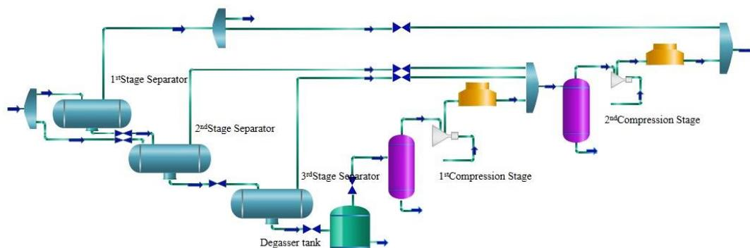
**Fig. A.6.** Schematic of crude oil production plant: The second method
