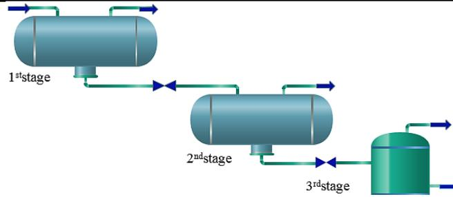
**Fig. A.3.** The schematic of Case#1 crude oil production plant using three separation stages
