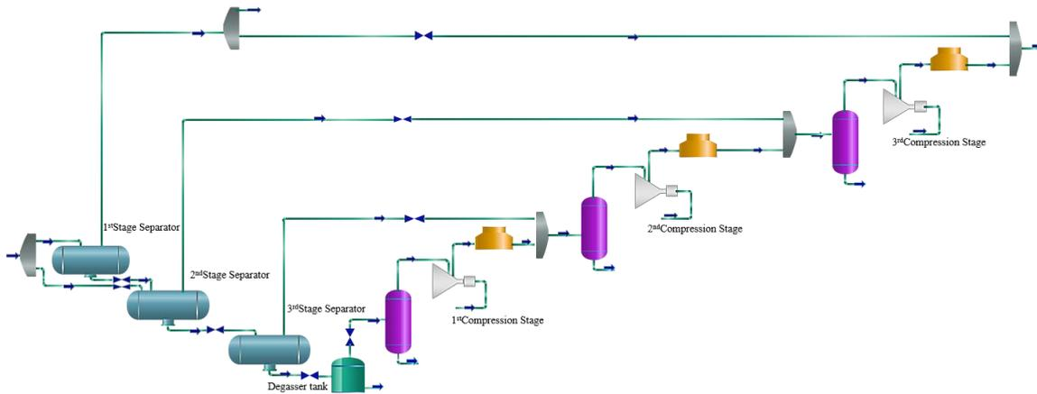
Fig. 4. The schematic of crude oil production plant: The first scenario
