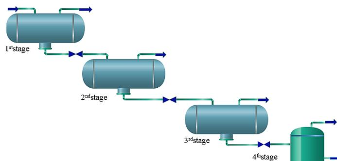
**Fig. 1.** The schematic of Case#1 crude oil production plant using four separation stages
