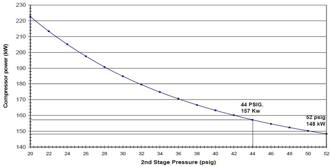
**Fig. A.5.** Effect of 2<sup>nd</sup> stage separator pressure variation on the compressors work
