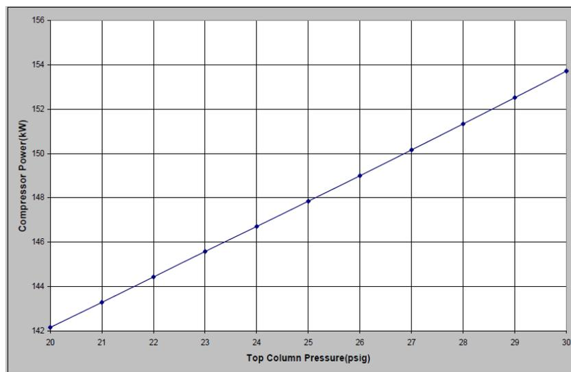
**Fig. A.11.** Compressor power vs. top column pressure variation
