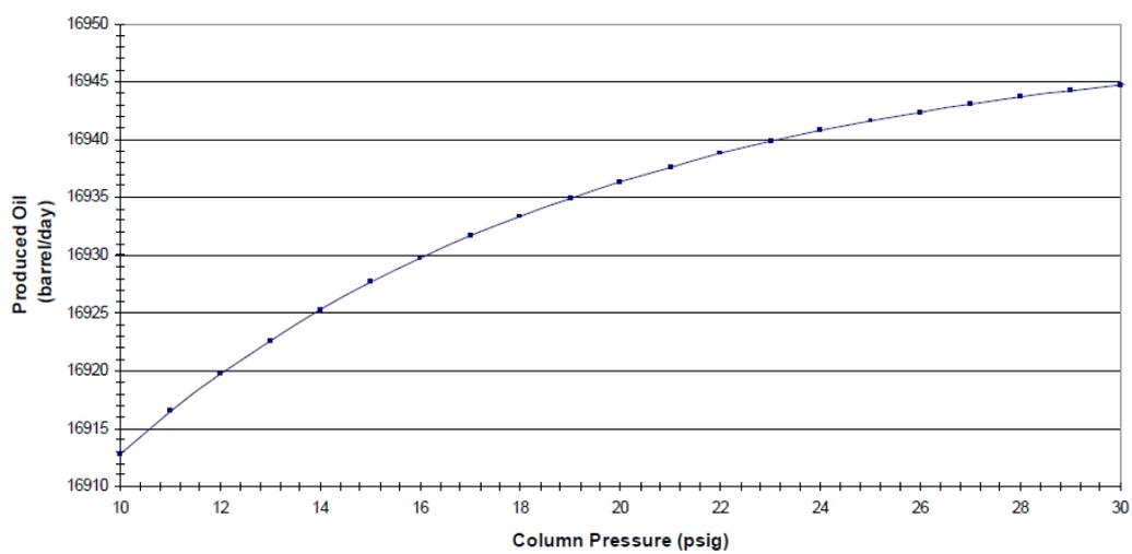
**Fig. A.12.** Effect of the stripping column pressure variation on the oil production rate
