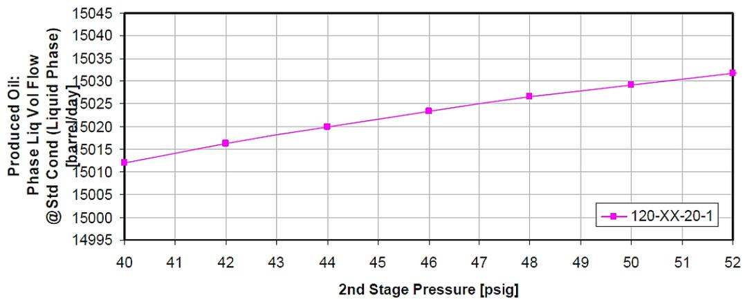
**Fig. A.1.** Changes in the Case#1 oil production rate versus 2<sup>nd</sup> stage separator pressure, assuming the 3<sup>rd</sup> stage separator pressure be 0.14 MPa
