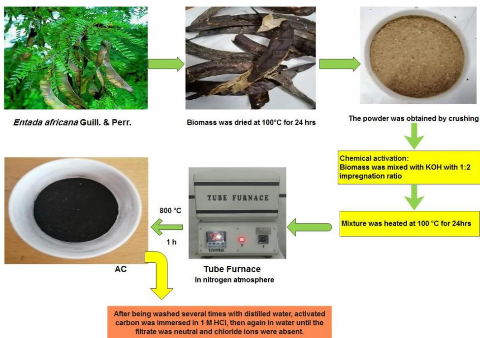
Fig. 1. The preparation steps of AC
