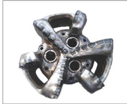
Figure 11: Centralized Nozzle arrangement
