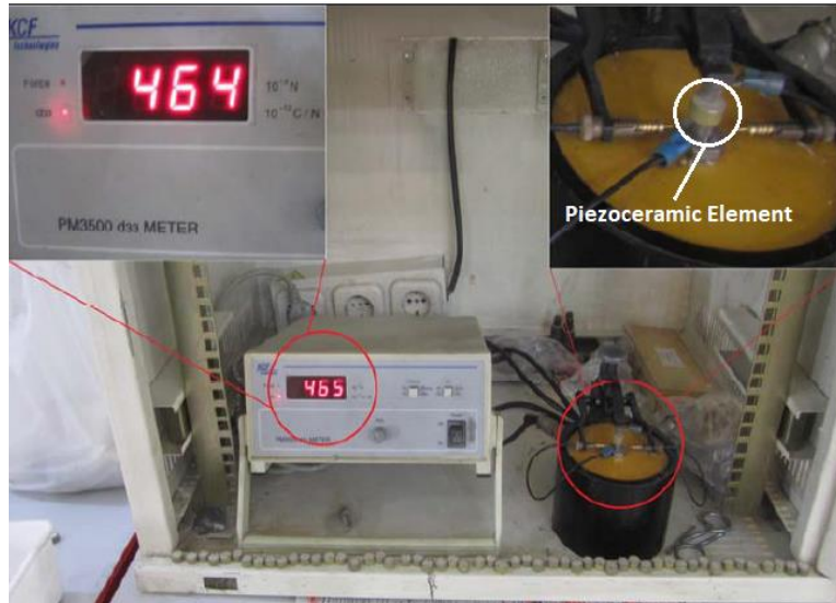
Fig. 3. Test setup for electrical impedance measurements
