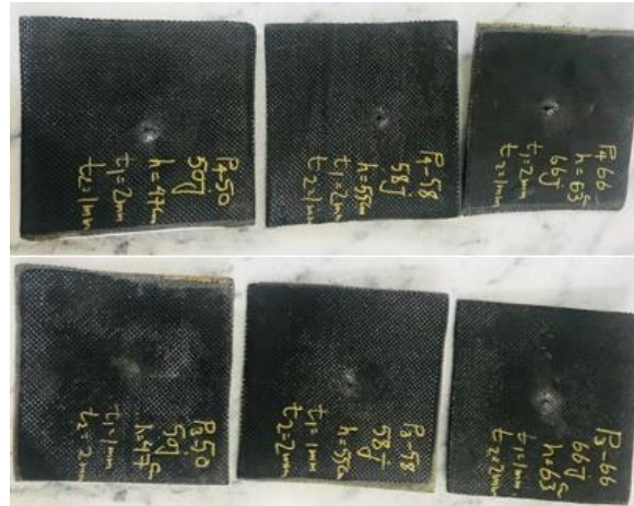
Fig. 20. Comparison of P501/2, P581/2 and P661/2 samples with P502/1, P582/1 and P662/ samples after impact test
