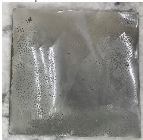
Fig. 2. The surface of aluminum after sandblasting process
