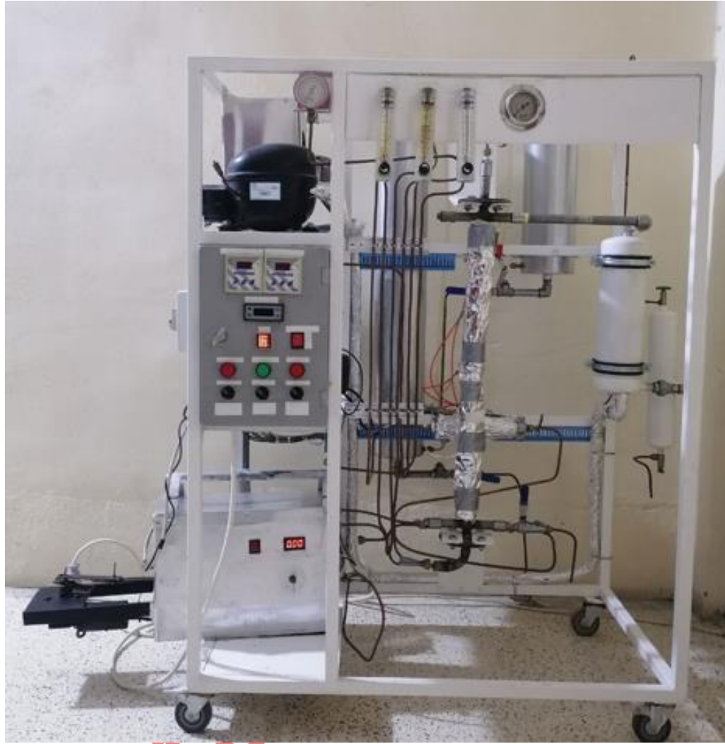
Figure1: Design of the oscillatory helical baffled reactor (OHBR)
