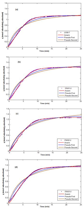
Figure 7: Comparison of kinetic models on experimental CO2 uptake vs. time for (a) UVM-7, (b) 5%N1-U, (c) 5%N2-U and (d) 5%N3-U
