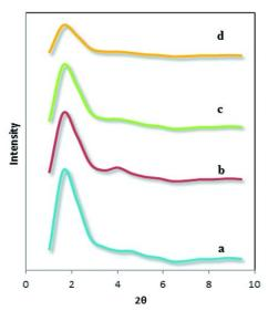
Figure 2: X-ray diffraction patterns of a) UVM-7 b) 5%N1-U c) 5%N2-U d) 5%N3-U
