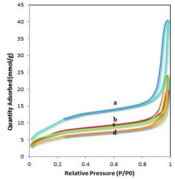
Figure 3: Nitrogen adsorption/desorption isotherms of a) UVM-7 b) 5%N1-U c) 5%N2-U d) 5%N3-U
